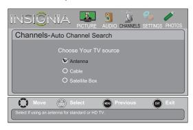
4 Press ▲ or ▼ to highlight Antenna, Cable, or Satellite Box, then press OK.
